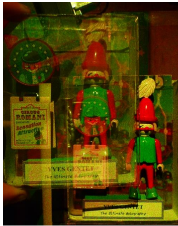
Figure 2. Original test object and hologram under a Red + Green laser beam light.
